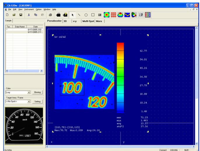
Advancement in display technology sees the rapid evolution of augmented reality head-up display that projects infotainment and enhance navigation information onto the windshield. Measuring of luminance and chromaticity in both night and day time is necessary to ensure consistent legibility.
