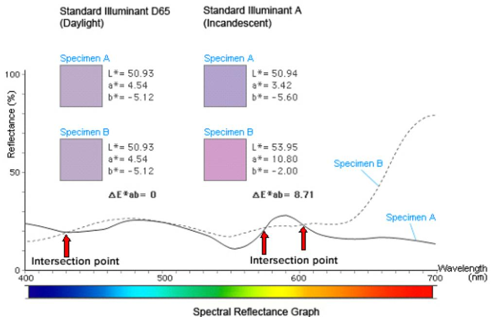
Figure 2 - Illuminant metamerism spectral reflectance curves
