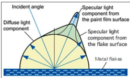
Figure 3 - Metallic coating reflection
