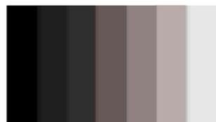
Intermediate red tone is strong here (The gamma value for R channel is lower as compared to G & B channel)
