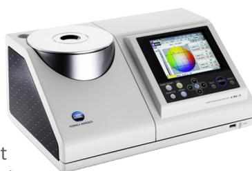
quality checks, development of products in research and development facilities and production processes. Chroma meter or spectrophotometer measure color using an integrating sphere. The sample is placed on the aperture of the integrating sphere and using a controlled illumination/light source to illuminate the sample, the light reflected by the sample is absorb and pick up by the sensor.
