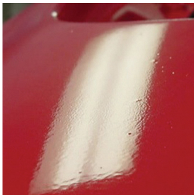
Figure 3 – Example of surface marked with orange peel
