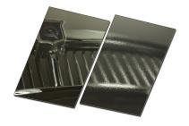
Orange peel is an effect that reduces the appearance quality without affecting gloss readings. As the name suggests, orange peel resembles the skin of an orange. Haze is a milky finish with a loss of reflected contrast. Halos and patterns can be seen around the reflections of high intensity light sources.
