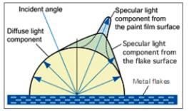
Figure 3 - Metallic coating reflection
