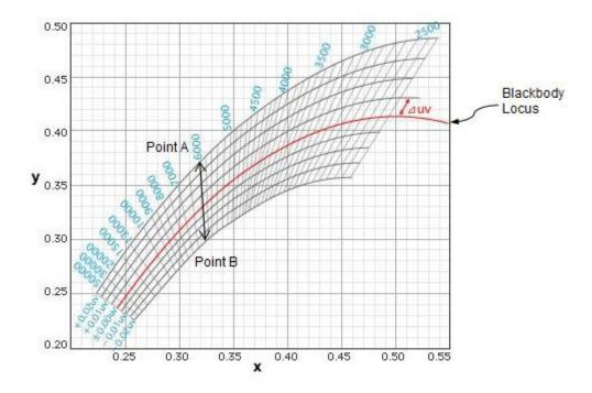
xy Chromaticity chart indicating the blackbody locus, the isotemperature lines and equal  $\Delta$ uv lines
