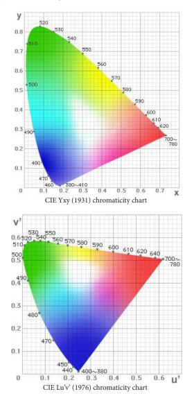
TThere are various color gamut standards drafted for expressing color display range according to different industry and different application. For smartphone and PC displays, the standard gamut is sRGB/ Rec.709. However, with the growing adoption of wide color gamut solutions in the high-end display market, wide color gamut standards such as Adobe RGB (used in high end digital cameras) and DCI-P3 (used in 4K Ultra HD TVs) are emerging as a key requirement for premium smartphone.
