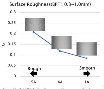
Figure 10 - TAMS<sup>™</sup> Surface Roughness Measurement Results Measurement of TAMS<sup>™</sup> also corresponds closely with the measurement of a white light interferometer (Wyko), as presented in Figure 11 and Figure 12.
