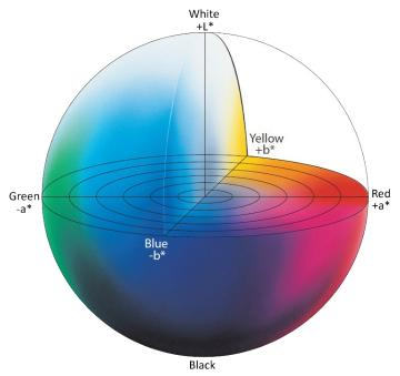
Figure 2 – Representation of color solid for  $L^*a^* b^*$  color space
