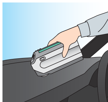
■ Spectrophotometer CM-2500c (Color management of components with different textures)
