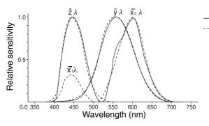
Fig. 1 Instrument's Spectral Sensitivity
