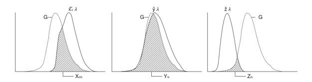
Fig. 3 Outputs of Sensors  $\overline{x}_2\lambda$ ,  $\overline{y}\lambda$ , and  $\overline{z}\lambda$  by Emitted Monochrome Light G
