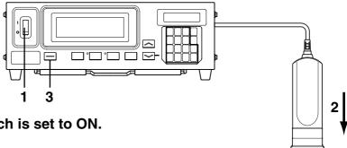
1. Check that the POWER switch is set to ON.
