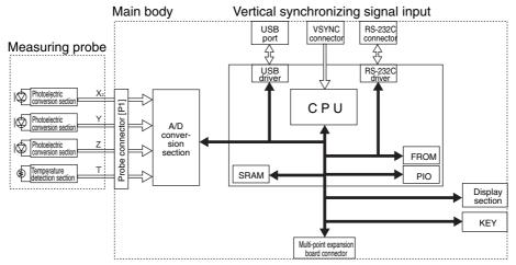
Fig. 2 Measurement Block Diagram
