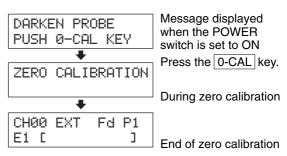
"E1" is always displayed if the instrument is used for the first time since shipment from the factory.
