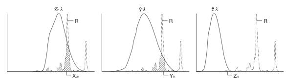
Fig. 2 Outputs of Sensors  $\overline{x}_2\lambda$ ,  $\overline{y}\lambda$ , and  $\overline{z}\lambda$  by Emitted Monochrome Light R
