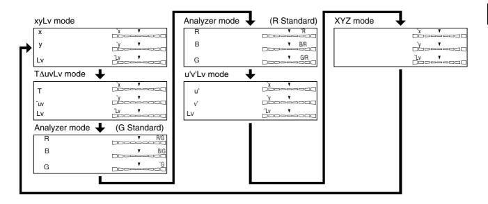
\* By default (factory setting), the instrument is set so that xyLv mode will be selected automatically when the POWER switch is set to ON. If you want to change this setting, refer to page 30.
