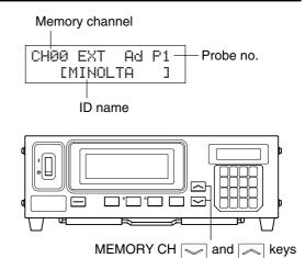
The desired memory channel can be selected by switching from one to another by pressing the MEMORY CH and keys.
