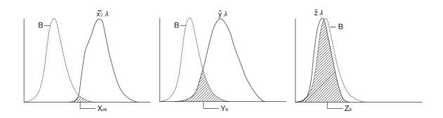
Fig. 4 Outputs of Sensors  $\overline{x}_2\lambda$ ,  $\overline{y}\lambda$ , and  $\overline{z}\lambda$  by Emitted Monochrome Light B
