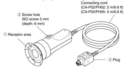
Measuring is done with a probe in intimate contact with the surface of display in the measuring part of this equipment. There are 2 m and 5 m long cord. There are 2 types of Measuring Probe.
