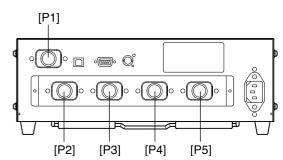
Connect necessary number of probes to the probe connectors [P2] to [P5] on the 4-Probe Expansion Board. You do not have to connect any probes to those connectors ([P2] to [P5]). Probes can be connected to any connectors ([P2] to [P5]).
