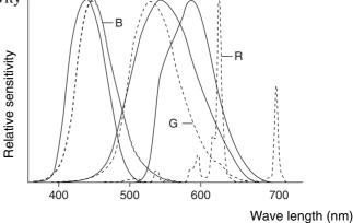
Fig. 1 Display's Spectral Distribution and Sensor's Spectral Sensitivity
