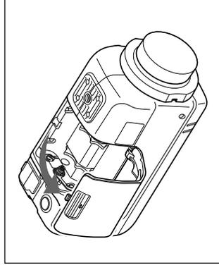
**3** Insert four AA batteries according to the polarity indications shown in the battery compartment.
