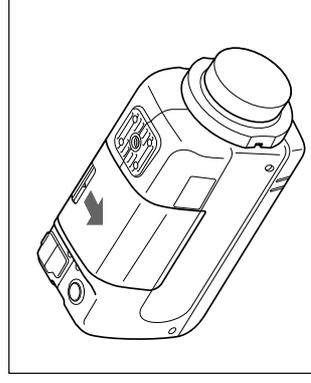
**2** To open the battery compartment cover, slide the cover in the direction indicated by the arrow.
