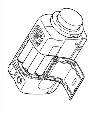
**4** To close the cover, insert the protrusions on the cover in to the holes on the battery compartment on the instrument, and then press the cover in until it clicks.
