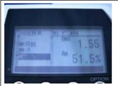
When the sample is measured, the solid density and dot area ratio is displayed.
