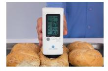
2. Using the PC application stored in the BC-10 Plus, you can set the instrument to store data internally (Memory capacity: 1000 data), transfer stored data to the PC, or take measurements from the PC.
