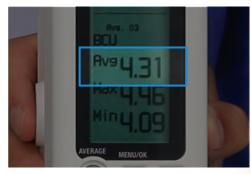
The BC-10 Plus takes as many measurements as required, and can store up to 16 readings at a time. To display the average of the stored readings, simply press the Average Button.
