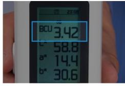
A Baking Contrast Unit is the measure of the lightness or darkness of a product. BCUs range from 0 for the darkest to 5.25 for the lightest. Each change of 0.1 BCU equals approximately on discernible shade to the human eye.
