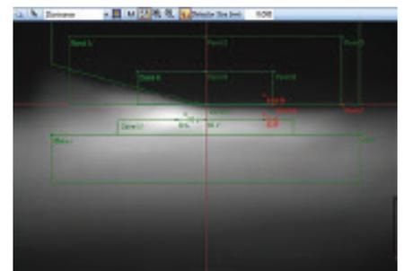
Figure 4 - Primary cut-off shape according UN ECE Regulation
