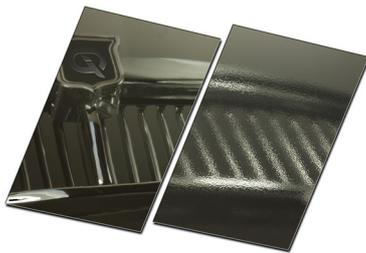
[Orange peel](#) is an effect that reduces the appearance quality without affecting gloss readings. As the name suggests, orange peel resembles the skin of an orange. Haze is a milky finish with a loss of reflected contrast. Halos and patterns can be seen around the reflections of high intensity light sources.
