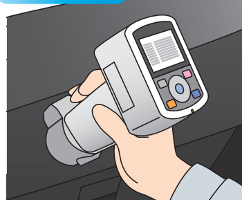
Spectrophotometer CM-700d (Color control of interior parts with curved surfaces and shapes)
