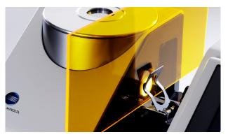
Plastic resins are also evaluated for yellowness and haze. Resins can vary from clear to cloudy or colorless to light yellow, amber and brown. During servicing, many resins turn yellow due to heat or the result of chemical degradation. For clear plastics, transmittance measurement of haze and yellowness are the two attributes commonly measured. For such measurement, a <u>sphere-based spectrophotometer</u> is recommended.
