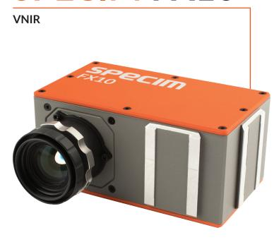
Specim FX10 camera series is designed for industrial and laboratory use. Specim FX10 cameras work in a line-scan mode in the visible and near-infrared (VNIR) area; Specim FX10 in the 400-1000 nm region, and the color optimized Specim FX10c camera in the 400-780 nm region.
